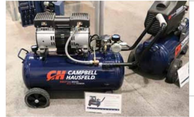
gap between DIY and the contractor market. Its 10-amp, 1-hp motor produces 125 psi at just 68 decibels. The company has also upgraded its large stationary units too.
