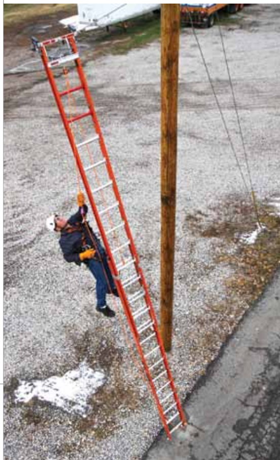
Little Giant Ladder Systems' Safety Cage ladder (below) has a full 360-degree wrap-around guardrail. The Claw Limited Fall Restraint (left) allows a user on the ground to securely fasten the top of an extension ladder to an overhead anchor point.
