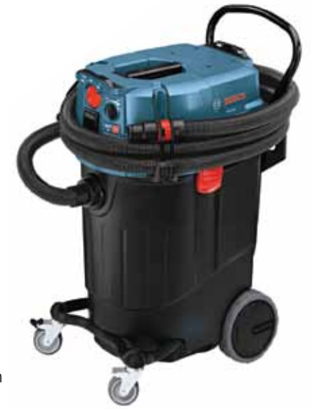
The 14-gallon Bosch VAC140A dust extractor self-cleans its filter through a reverse airflow every 15 seconds during operation without compromising suction or performance.
