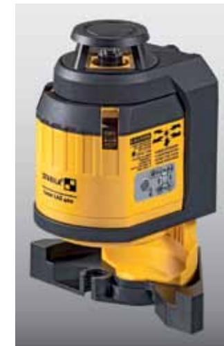
The LAX 400 Pro Liner multi-line self-leveling laser from Stabila has a working range of 60 to 490 feet with receiver, and works with or without a receiver. It produces bright, crisp lines and dots including a 360-degree horizontal line, two vertical lines at 90 degrees to each other and plumb points.
