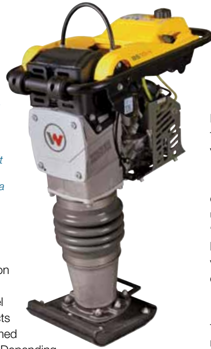
Wacker Neuson's largest rammer is the model BS70-4As. Powered by a 3.6-hp four-cycle Honda GXR120 engine, it weighs 177 pounds and produces 678 bpm with a 2.9-inch shoe stroke.
