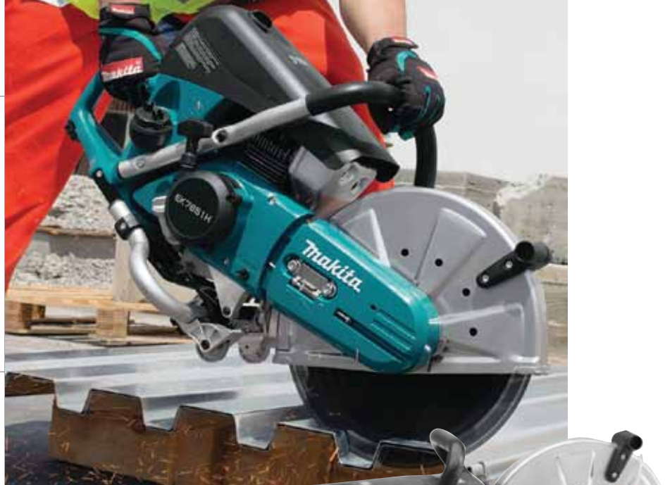
Makita's 14-inch model EK7651H is the world's first power cutter with a four-cycle engine that eliminates the need to mix gas and oil. It also boasts easy starts, lower noise and better fuel economy.
