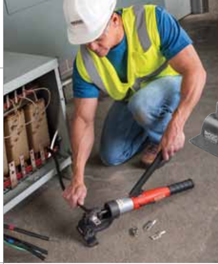
The RIDGID RE 12-M manual hydraulic crimp tool has a 1.65-inch jaw opening and can produce crimps up to 1,000 MCM and has a 330-degree rotating head for access in tight spaces.
