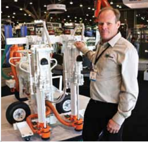
At Left, Minnich Manufacturing's Rob Minnich displays the company's new OSHA-compliant venturi vacuum dust collection systems for dowel pin drills. Dust is collected into pails that can be quickly swapped out and disposed of properly later.
