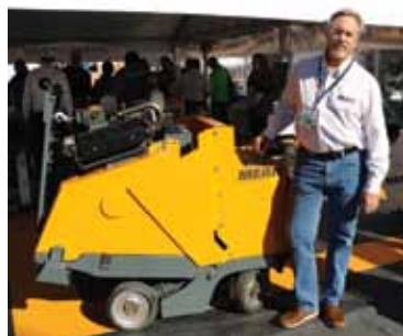
Below, Merit Engineering & Equipment vice president Greg Ferguson displays the industry's first all-wheel drive steerable concrete saw.
