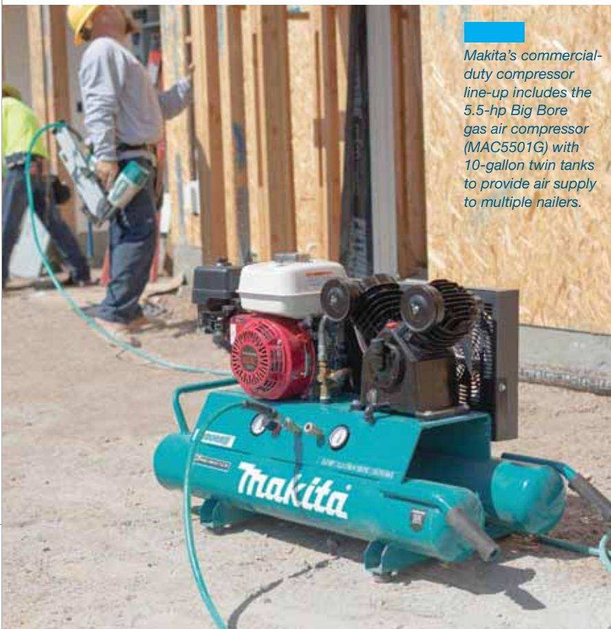
Makita's commercial-duty compressor line-up includes the 5.5-hp Big Bore gas air compressor (MAC5501G) with 10-gallon twin tanks to provide air supply to multiple nailers.
