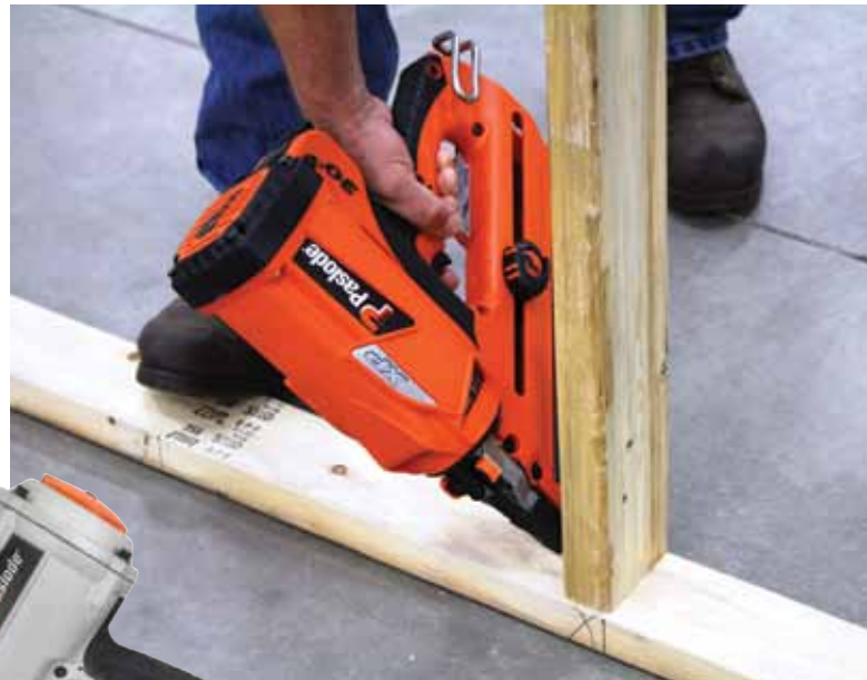
Above: Paslode's Cordless XP Framing Nailer has 15 percent more power to drive nails flush even into LVL. Left: The Powermaster Pro Framing Nailer weighs 7.9 pounds, 1/2 pound less than its predecessor.
