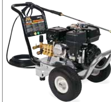
WP-3200-0MHB - 3200 PSI @ 2.4 GPM - Direct drive triplex piston Mi-T-M pump - 196cc Honda GX200 OHV engine
