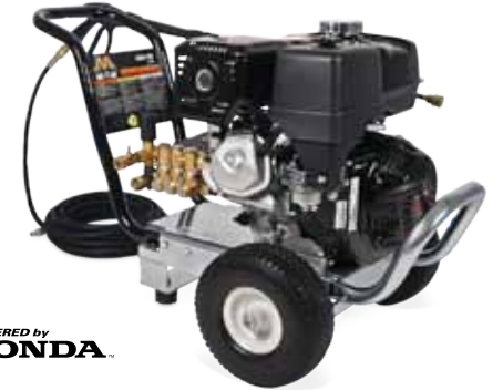
WP-4200-0MHB - 4200 PSI @ 3.4 GPM - Direct drive triplex piston AR pump - 389cc Honda GX390 OHV engine
