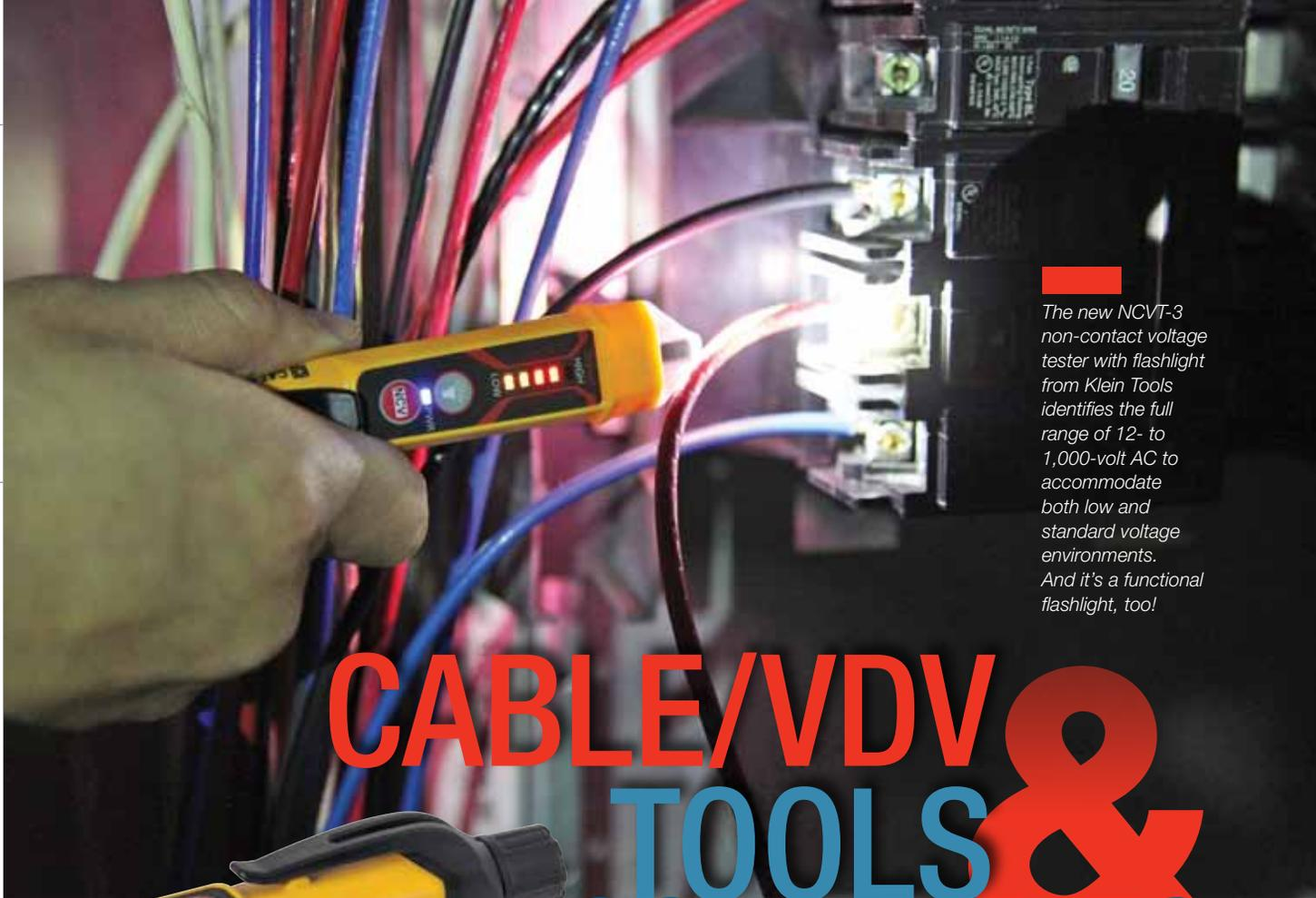
The new NCVT-3 non-contact voltage tester with flashlight from Klein Tools identifies the full range of 12- to 1,000-volt AC to accommodate both low and standard voltage environments. And it's a functional flashlight, too!
