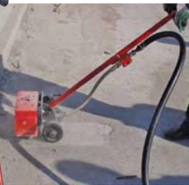
CS Unitec's Trelawny MHS11 multi-headed concrete floor scabbler produces seven times less vibration than standard models thanks to a three-point mechanical vibration damping system.
