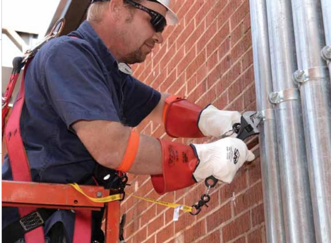
In Snap-on Industrial's Tools at Height tethered tool line, tethers are not added as an after-thought, but are engineered into the tool to maintain or improve the functionality of the tool when tethered.
