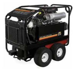
Mi-T-M's mighty new AR1-PK37-M rotary screw compressor produces 115 cfm at 100 psi, plenty of air to power a 90-pound breaker hammer. It has a 10.5-gallon aluminized steel fuel tank and a full set of durability features.
