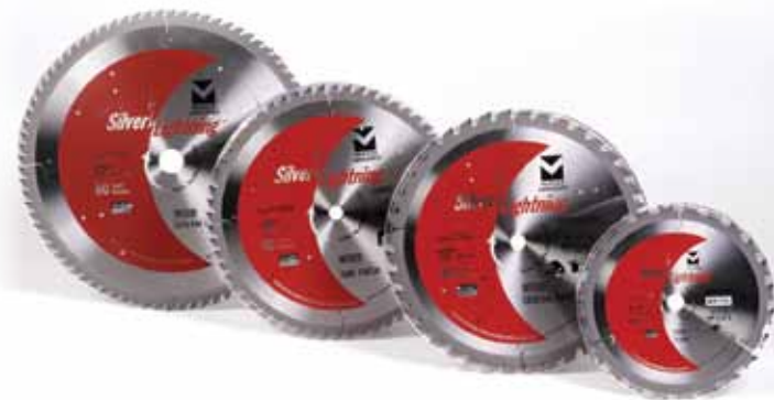
Mercer Silver Lightning blades are available with either alternate top bevel (ATB) teeth for circular saws cutting wood, Hi-ATB teeth for miter and table saws for knife edge cuts or Triple Chip Grind for miter and table saws cutting hard materials.
