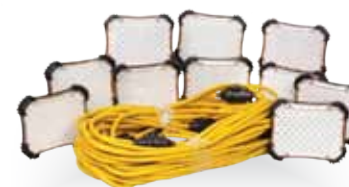
100' LED String Lights with Slide Lock Connection - Daisy chain up to 750 continuous feet on a 20 amp circuit - 18/2 STW cord with 6w, 680 lumen panels spaced 10' apart
