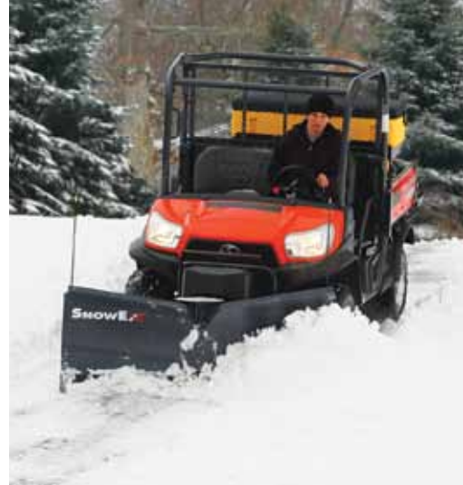
The SnowEx V-Plow for UTVs measures 6 feet wide and can assume straight, "V" or bucket blade scoop positions for optimum performance on sidewalks and through gates.
