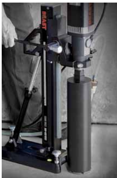
Lackmond's model BCR300/12 mast mounted core drill rig's three-speed, 3.2-horsepower motor can drill holes up to 12 inches in diameter. Its LED amp meter helps ensure optimum drilling pressure.
