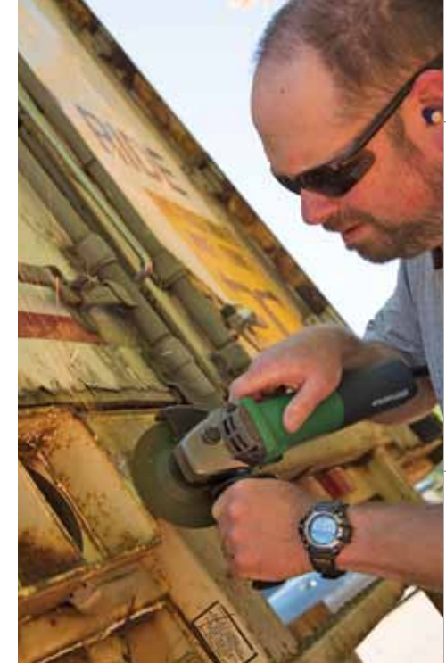
Safety features of the Hitachi G12VE AC brushless grinder include electronic overload protection, anti-kickback protection, soft start and zero-voltage restart.
