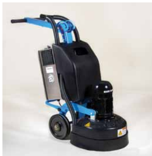
The Innovatech model P1800 grinder polisher from Bartell Morrison features a three-head planetary design for rigid or flexible seven-inch heads. It has a single-phase 208-240 volt, four-hp motor.
